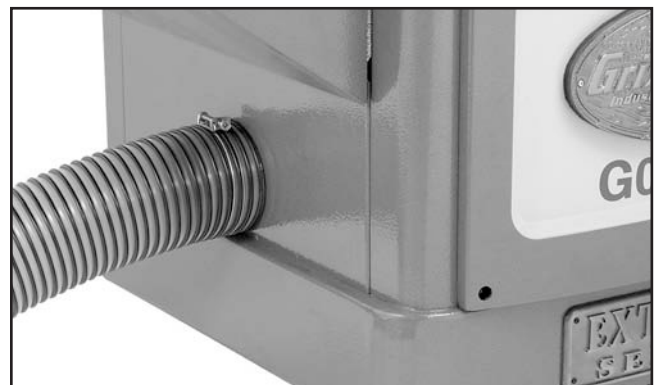
Figure 34. Dust hose attached to dust port.
